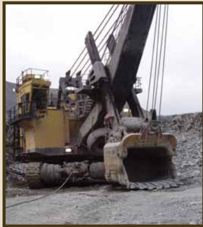
Trailing cables are used throughout the industry even in surface operations.
