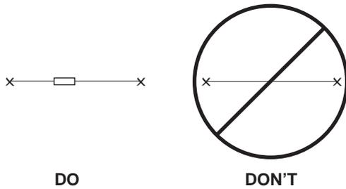
permit, the guides on one side of the expansion compensation device can be eliminated by locating the unit adjacent (within 4 pipe diameters) to an anchor.
