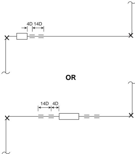
At the system designers option, some long straight pipe runs may require additional guides to maintain pipe alignment and prevent "bowing" and pipe joint deflection on areas remote from the expansion compensation device. The use of Victaulic Style 07 Zero-Flex® rigid couplings with proper pipe support spacing (see Victaulic publication 26.01 for additional information) may eliminate the need for the additional guides.
