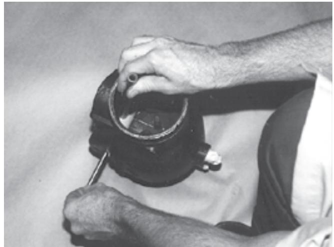
8. While holding the tool with one hand, insert the new shaft (provided in the kit) into the valve. Pass the shaft through the disc, torsion spring, and into the other side of the valve body.
