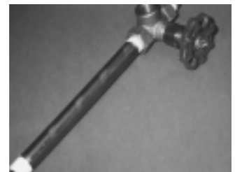
Step 8: Assemble the 1/2" X 6 1/2" (15 X 165 mm) long nipple (Item #6) and the 1/4" pipe plug (Item #7) to the remaining 1/4" NPT three way globe test valve (Item #2) using a suitable teflon tape or pipe dope.
