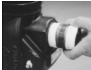
Step 3: Install the 2" (50 mm) nipple (Item #4) in the Series 717R valve body.
