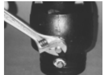
Step 4: Remove both 1/4" (6.4 mm) NPT pipe plugs.
