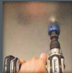
Drill and deburr hole in freezer bracket
