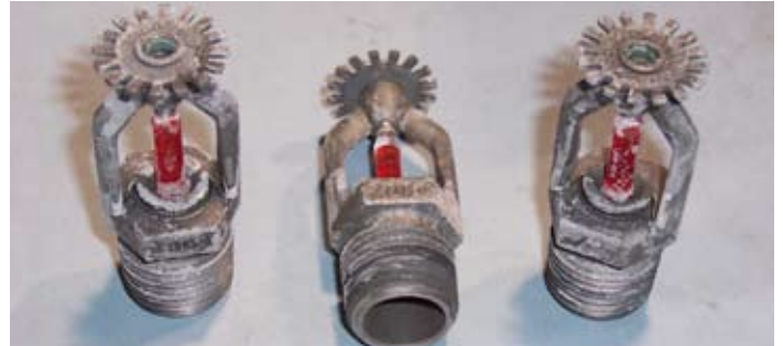
Proprietary Nickel-Teflon coated Victaulic sprinklers after 30 day 20% salt Fog
