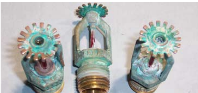
Plain Brass finished Victaulic sprinklers after rinse
