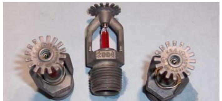
Proprietary Nickel-Teflon coated Victaulic sprinklers after rinse
