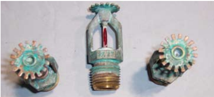
Plain Brass finished Victaulic sprinklers after 30 day 20% salt Fog
