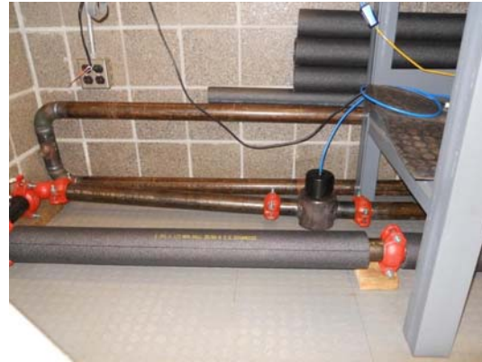
Picture 3 Oxygen probe
