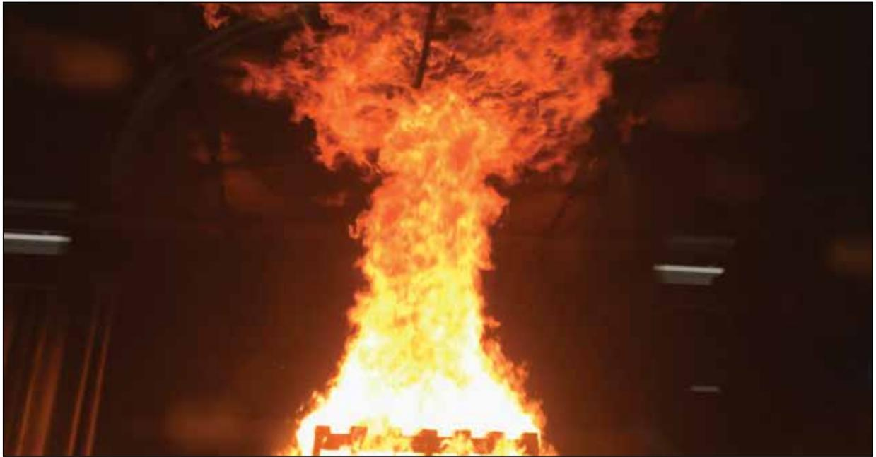
Victaulic FireLock™ Installation-Ready™ Fittings put to the test by UL, LLC in the United States, as part of the certification requirements for mechanical joints used in dry pipe fire protection systems in buildings and facilities.
