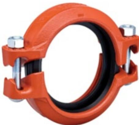
Victaulic couplings are advanced mechanical pipe joining components engineered to provide a secure, leak-tight seal. Designed to withstand system movement, including hanging loads and bending forces, these couplings also offer flexibility for thermal expansion and contraction when required. Each coupling consists of two or more high-strength ductile iron housings, a resilient elastomer gasket, and a set of engineered fasteners to ensure reliable and efficient assembly.
